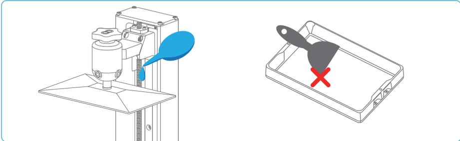
3. Be careful when you remove the build platform in case you may damage the tempered glass or screen.
