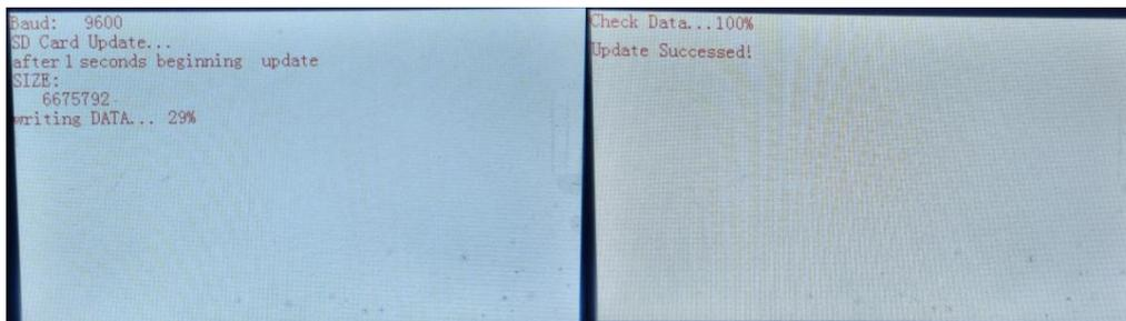
After loading is complete, you **must remove the TF card** and then restart the machine.
